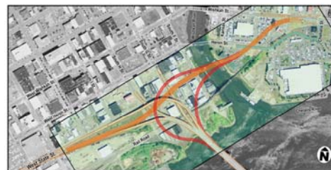
The new US 12/US 101 interchange would provide ramps from northbound US 101 to eastbound US 12 and from westbound US 12 to southbound US 101.
